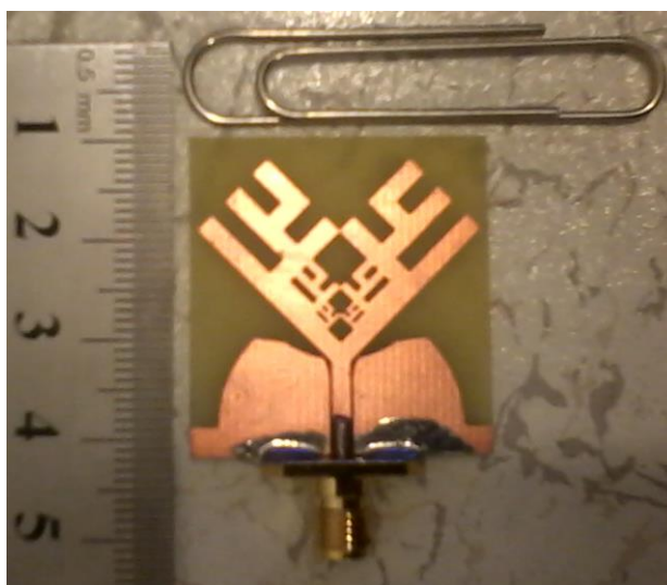
Figure 16. The photograph of the proposed realized antenna.
